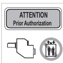
It's compulsory to request HYDRO-MEC authorization to use our gearboxes when the units are used in a man lift or people moving devices.
