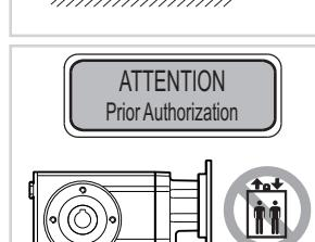
It's compulsory to request HYDRO-MEC authorization to use our gearboxes when the units are used in a man lift or people moving devices.
