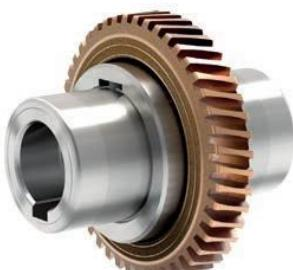
**Nickel bronze worm gears CuSn12Ni (C91700) is centrifugally cast onto an iron hub for maximum strength and superior life.**
