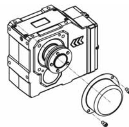
Fig. 10: Protection cap for shrink disc hollow shaft
