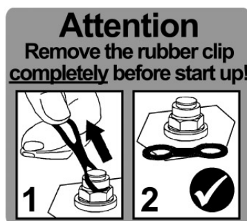
Fig. 2: Information label (red) on the gear unit
