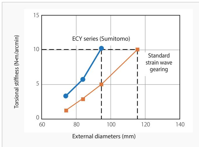
The torsional stiffness is approximately twice that of a standard strain wave gear (same size), which results in a stronger unit with considerably reduced vibration.
