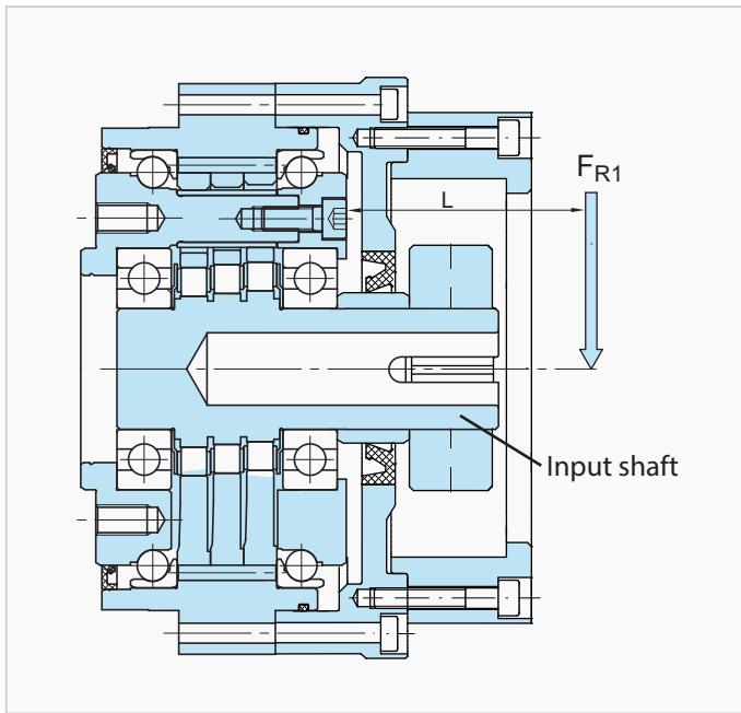
Fig. DA-4 Load position on input shaft
