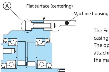
The Fine Cyclo C Series is attached to the machine casing by bolts. (spigot Z)
