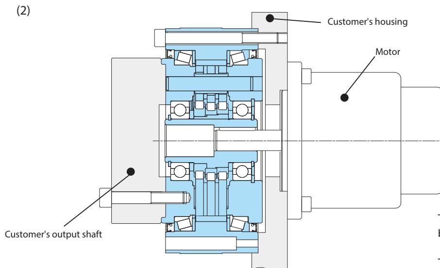
The motor and the Fine Cyclo F2C-A gearbox are both bolted onto the customer's housing.
