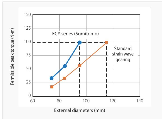
The permissible peak torque is approximately 1.5 times higher than that of a standard stress wave gear (same size), which means that the gearbox can be more compact.
