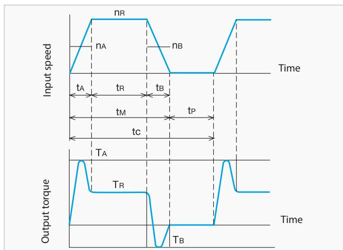
The load cycle ( $t_c$ ) reflects the sequence of movements in the application used. This typically consists of at least one acceleration phase ( $t_A$ ), one constant speed phase ( $t_R$ ), one deceleration ( $t_B$ ), and one pause of movement ( $t_p$ ).
