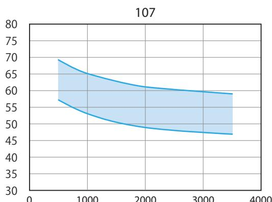
Fig. ECY-3 Efficiency of E Cyclo 107
