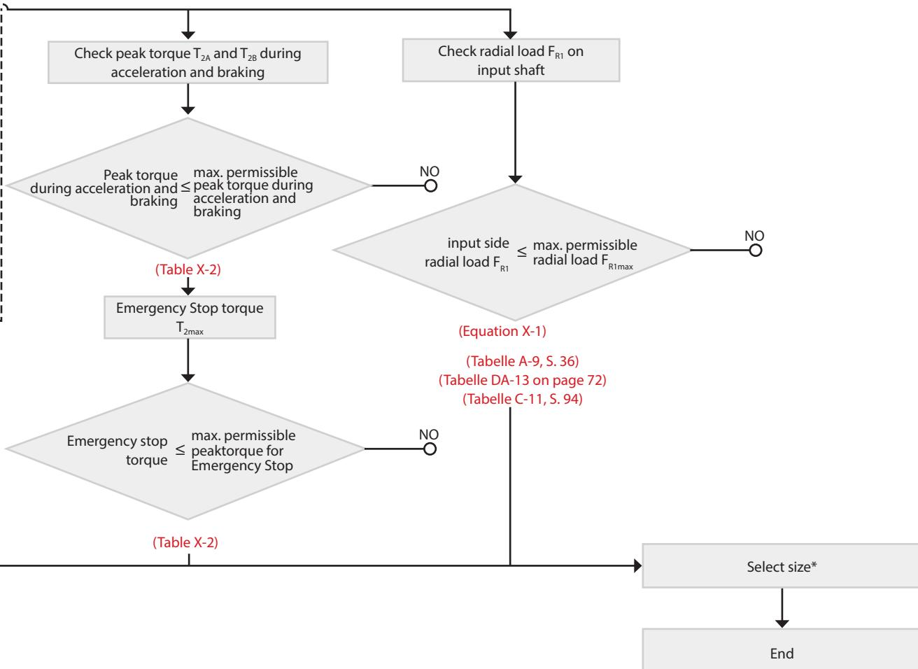
\* When selecting the motor, the input side breakaway torque (BTI) or no-load running torque (NLRT) must be taken into account.
