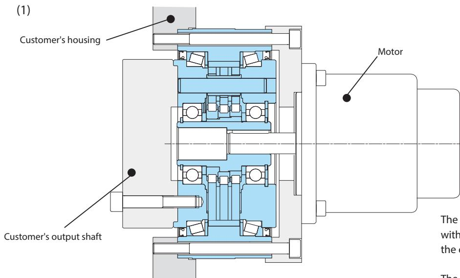
The motor is connected via an intermediate flange with the Fine Cyclo F2C-A gearbox and bolted onto the customer's housing.
