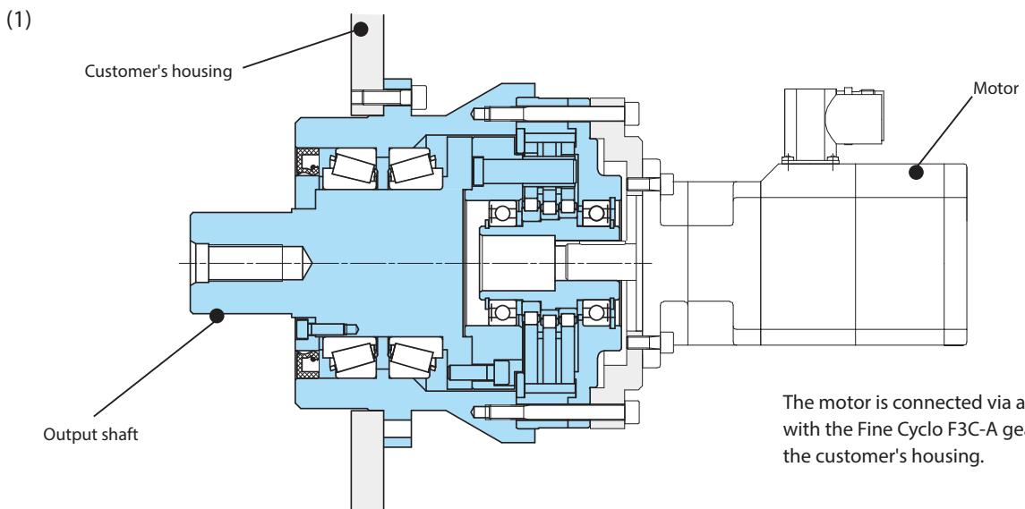
The motor is connected via an intermediate flange with the Fine Cyclo F3C-A gearbox and bolted onto the customer's housing.
