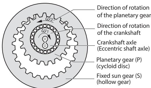
Fig. 1 Principle of the internal planetary gearbox
