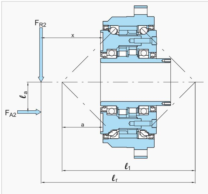
Fig. C-5 Distance between the individual loading points
