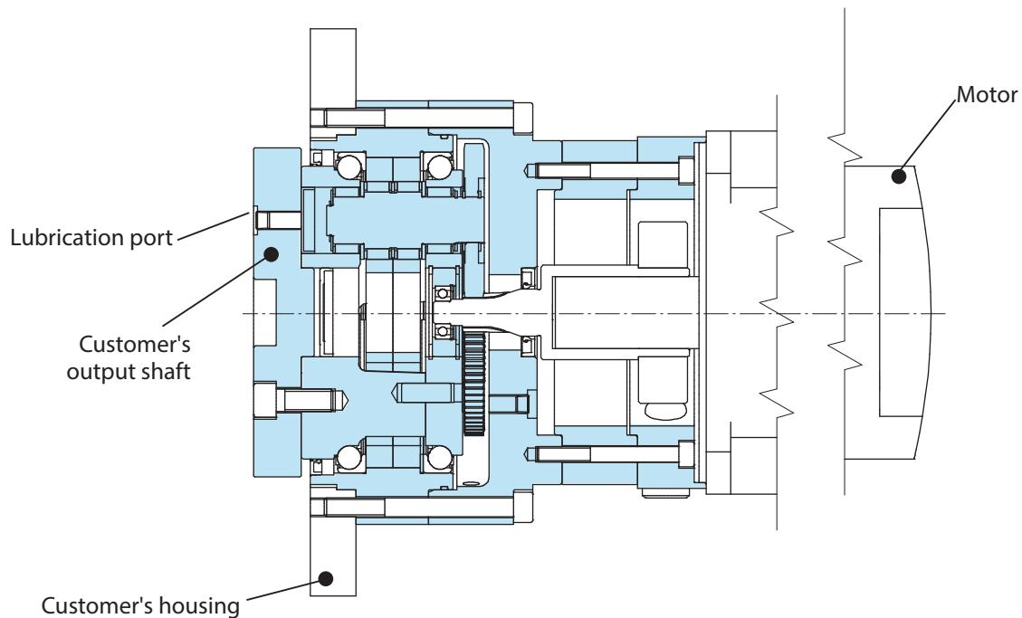
The customer's output shaft is bolted to the output flange of the gearbox.
