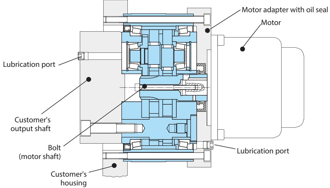
An adapter is required for the installation of the motor on the input side flange. This can be supplied. An oil seal must be provided in this adapter. The input shaft of the gearbox is not mounted in the gearbox.
