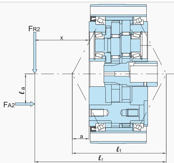
Fig. T-4 Distance between the individual loading points
