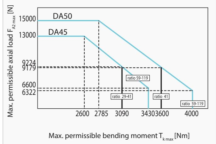
Fig. DA-6 Max. permissible bending moment and axial load
