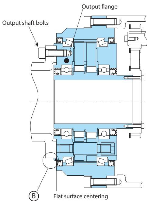
Use bolts to attach output flange of Fine Cyclo to output shaft of machine.
