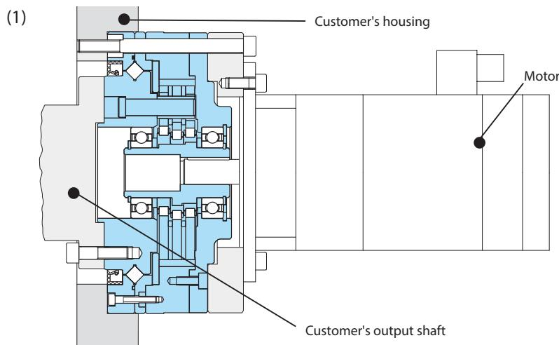
The motor is connected via an intermediate flange with the Fine Cyclo F1C-A gearbox and bolted onto the customer's housing.
