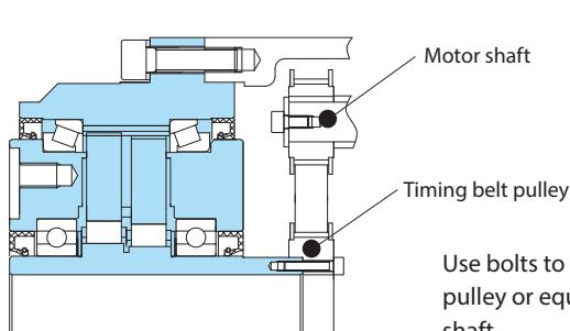
Use bolts to attach the timing belt pulley or equivalent parts to the input shaft.
