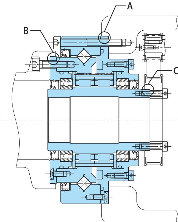
Fig. ECY-8 Installation of E CYCLO
