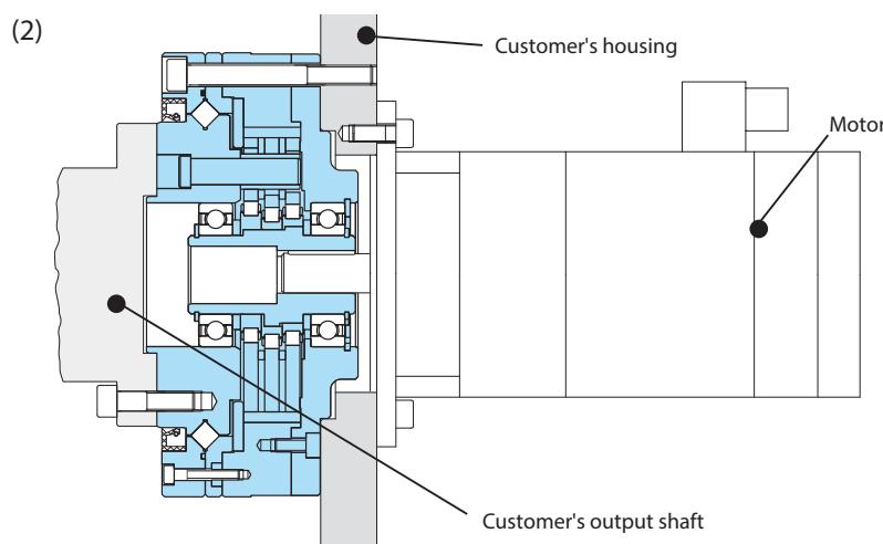
The motor and the Fine Cyclo F1C-A gearbox are both bolted onto the customer's housing.
