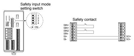
To connect the safety sensors, set the semiconductor input mode (switch No. 1 and 3 to OFF and switch No. 2 and 4 to ON) and open the circuits between SI+ and SO+, and between SI- and SO-. Safety sensors can be connected to this device.
