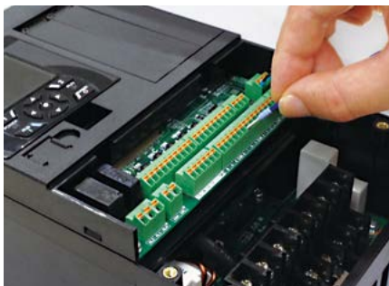
Screwless terminal block (control terminal block).
