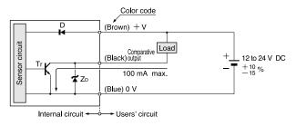
Symbols ... D : Reverse supply polarity protection diode Zo: Surge absorption zener diode Tr: NPN output transistor
