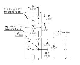
Material: Cold rolled carbon steel (SPCC)
