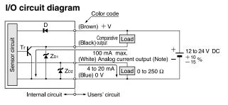
Note: The analog current output does not incorporate a short-circuit protection circuit. Do not connect it directly to a power supply or capacitive load.
