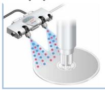
Removing charges during pickup from dicing tape
