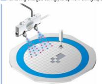
Removing charges from LCD module clamps
