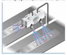
Removing charges during cell production
