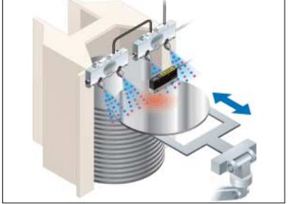
Measurement of lead frame charge removal
