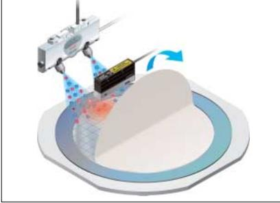
Surface potential measurement during chip release electrification
