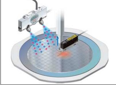
Surface potential measurement during loading and unloading
