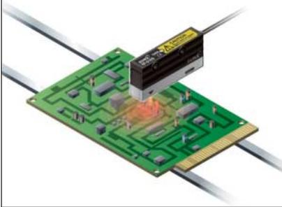
Measurement of frictional electrification of LCD modules
