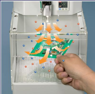
Direct ion emission paired with pulsed air emission provides quick and effective removal of static charges along with any dust that is present on the part.
