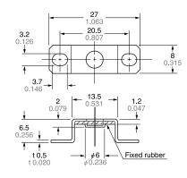
Material: Bracket ... Stainless steel (SUS304) Fixed rubber ... FKM (Fluorine rubber)
