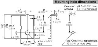
Material: Cold rolled carbon steel (SPCC) (Nickel plated)
