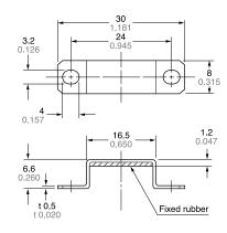
Material: Bracket ... Stainless steel (SUS304) Fixed rubber ... FKM (Fluorine rubber)
