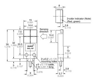
Note: Normally closed DC 2-wire type, NPN output type and PNP output type have an operation indicator (red) instead of the 2-color indicator.
