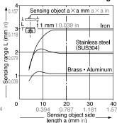
As the sensing object size becomes smaller than the standard size (iron sheet  $20\times20\times t$  1 mm  $0.787\times0.787\times t$  0.039 in), the sensing range shortens as shown in the left figure.
