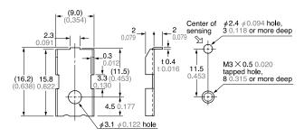
Material: Cold rolled carbon steel (SPCC) (Nickel plated)
