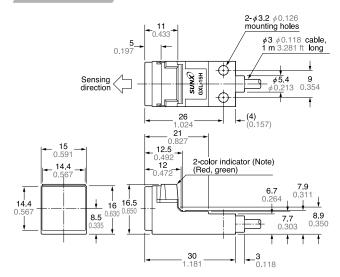
Note: Normally closed DC 2-wire type and NPN output type have an operation indicator (red) instead of the 2-color indicator.
