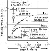
As the sensing object size becomes smaller than the standard size (iron sheet  $30 \times 30 \times t$  1 mm  $1.181 \times 1.181 \times t$  0.039 in), the sensing range shortens as shown in the left figure.
