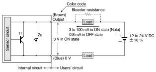
Symbols ... Zp: Surge absorption zener diode Tr: PNP output transistor
