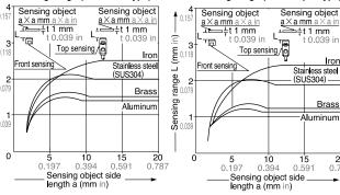
As the sensing object size becomes smaller than the standard size (iron sheet  $15\times15\times t$  1 mm  $0.591\times0.591\times t$  0.039 in), the sensing range shortens as shown in the left figures.
