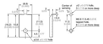
Material: Cold rolled carbon steel (SPCC)
