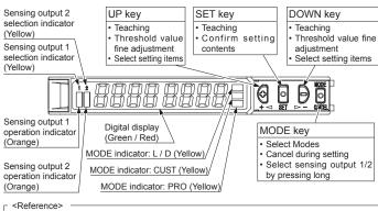
Pressing down SET key + MODE key for 3 sec : Set key lock or Release key lock
