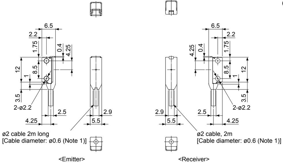
Note: The cable diameter of inflection resistant cable type is  $\varnothing 0.7$ mm.
