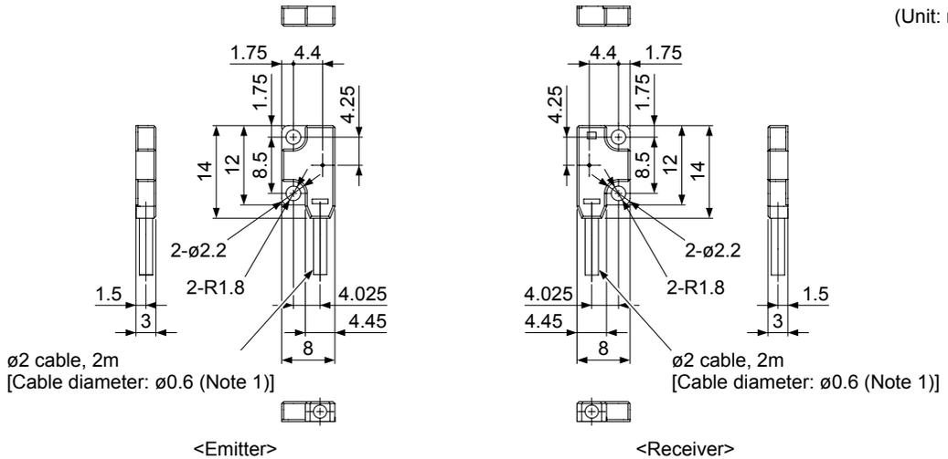
Note: The cable diameter of inflection resistant cable type is  $\varnothing 0.7$ mm.
