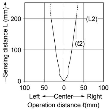
In case using at sensing distance (L2) 200mm, the operation point (ℓ2) is approx. 30.5mm according to the diagram at left.
