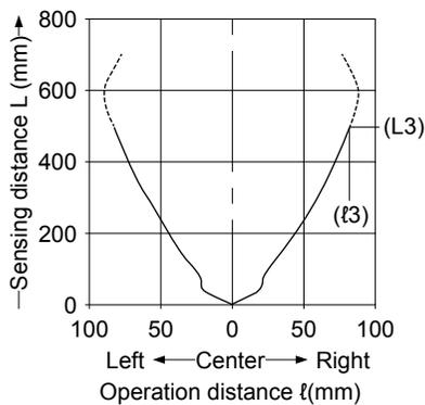
In case using at sensing distance (L3) 500mm, the operation point (ℓ3) is approx. 81.9mm according to the diagram at left.
