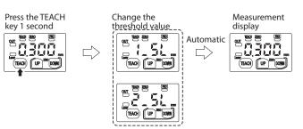
When performing a fine adjustment of the threshold of  $\frac{1}{2}$  or  $\frac{2}{2}$  or  $\frac{2}{3}$ , press the UP key or DOWN key. After  $\frac{1}{2}$  or  $\frac{2}{3}$  is displayed, the fine adjustment of the threshold can be performed.
