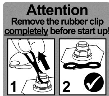
Fig. 3: Information label (red) on the gear unit
